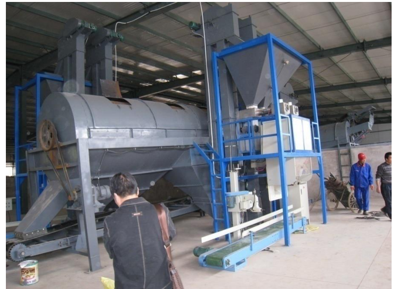
Post treatment equipments: crusher, siever and conveyor belts
