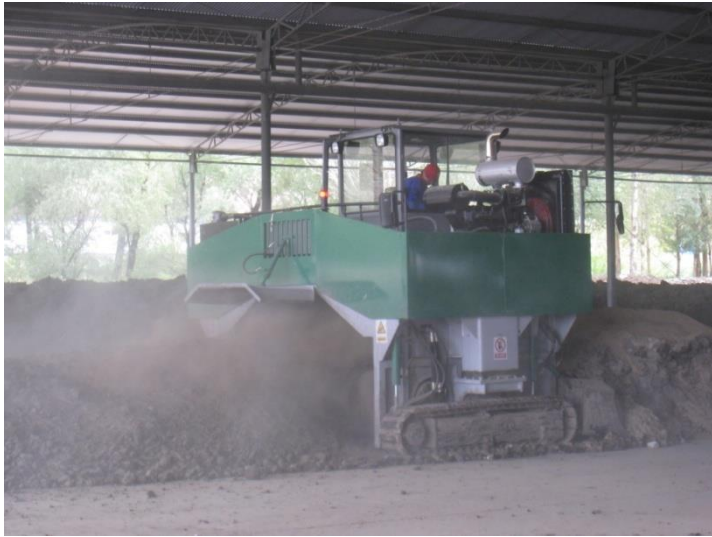
Indoor composting area and compost turners
